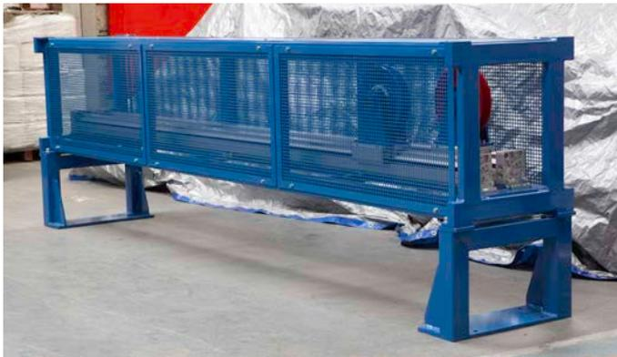
*Picture shows the horizontal tensioner with close guarding bolted to both sides. This shot was taken just before the unit was shipped to the client.*
